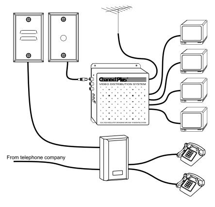
A ChannelPlus DoorTel system (model 9400) is an ideal addition to this system. In this house, when the doorbell rings, the homeowner changes the TV to the front door channel and picks up any phone in the house. The homeowner can talk with and see the guest at the front door.
